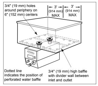
Figure 4. Hydro-Heater Water Baffle
